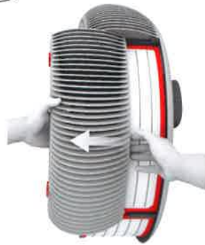
Slide out the inlet grilles
